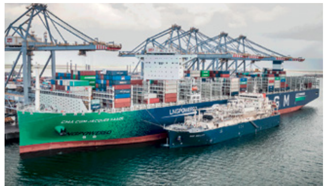
Gas Agility and CMA CGM Jacques Saade participating in the world's largest LNG bunkering operation, a transfer of 17,300 m 3 of product, in Rotterdam in November 2020
