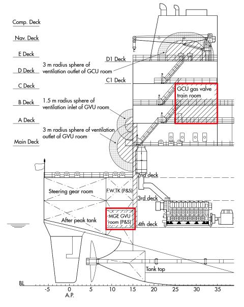
Figure 3: Gas valve room is a hazardous area
