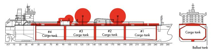
Figure 1: Hazardous area on an LPG carrier
